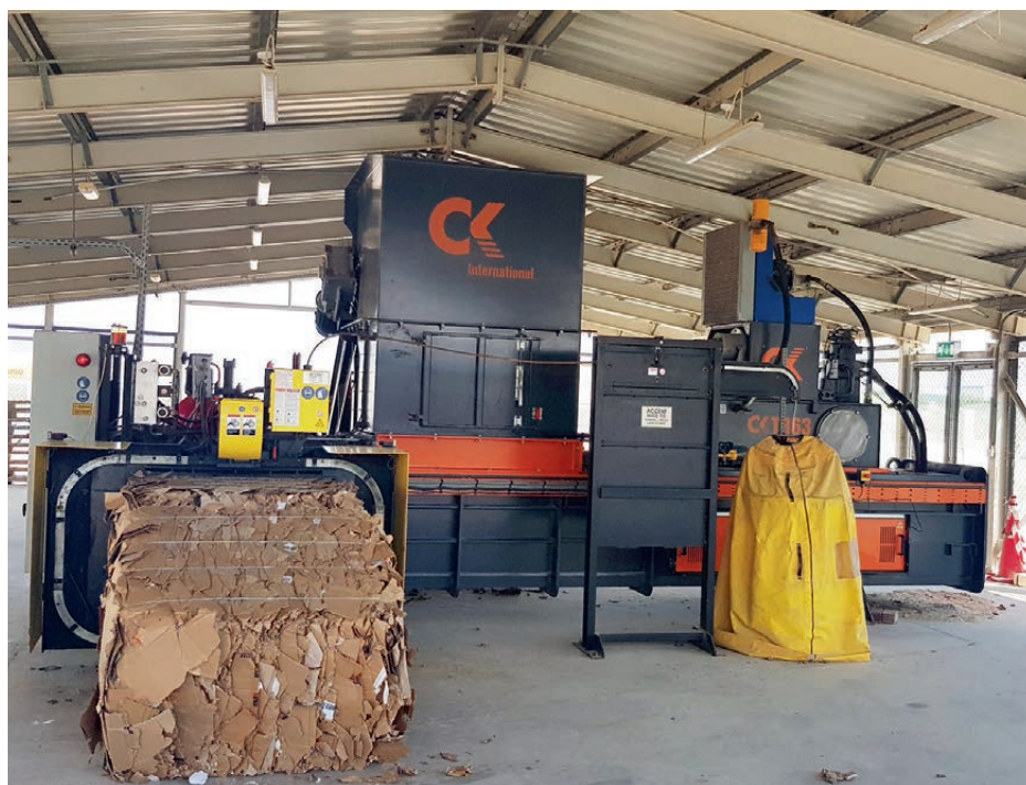
CKTR63-60T-22kW Twin Ram Baler processing cardboard waste
