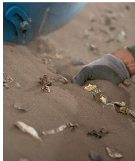
SandFlo™ uses aerated sand to sort secondary metals by density
