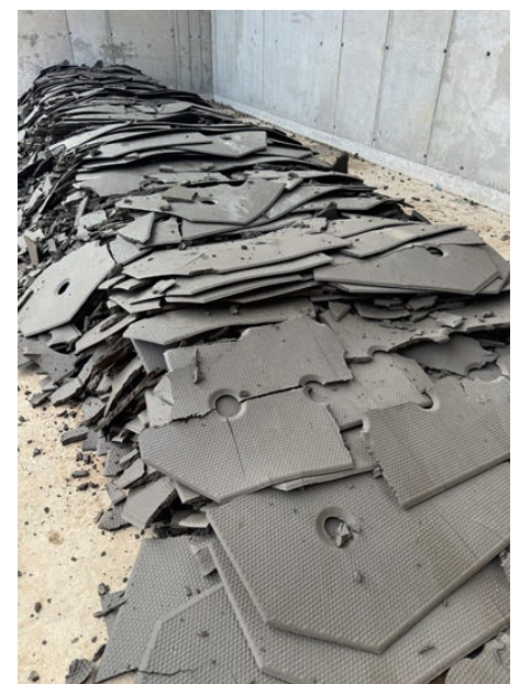
The pressed silt cakes produced by SunAggregates' new filter press at their site in Thetford
