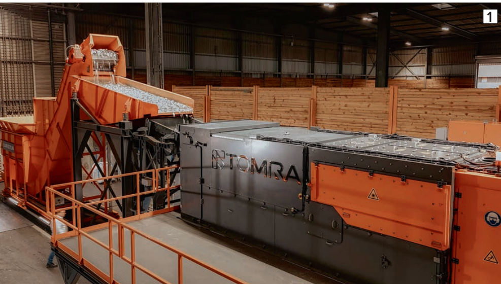
1. TOMRA's AUTOSORT™ PULSE now allows Gerhard Lang Recycling GmbH to produce high-purity 5xxx and 6xxx aluminium scrap. 2. At the core of the system is TOMRA's Dynamic LIBS solution, an in-house developed, advanced laser technology that separates the alloys based on the elemental composition. 3. The purity levels that Gerhard Lang Recycling achieves exceed 95% and can potentially reach 97%, making the material suitable for use in the production of aluminium without downgrading
