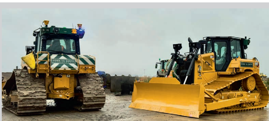
Down to Earth Developments bought two electric-drive Cat D6 XE dozers last year from Finning UK and Ireland
